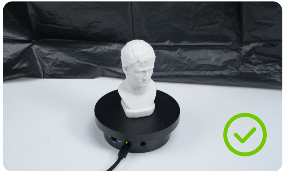
Using Magic Mat or black bin bag as the background, and ensuring consistent and even illumination.
